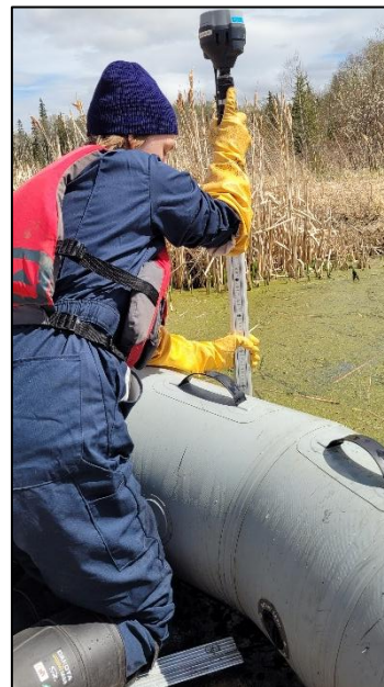
Figure 6 Liner measurements taken using a GNSS mounted survey rod (sample image)
