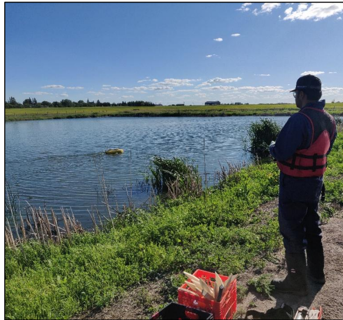
Figure 3 Hydrasurvey inshore survey vessel on survey (sample image)
