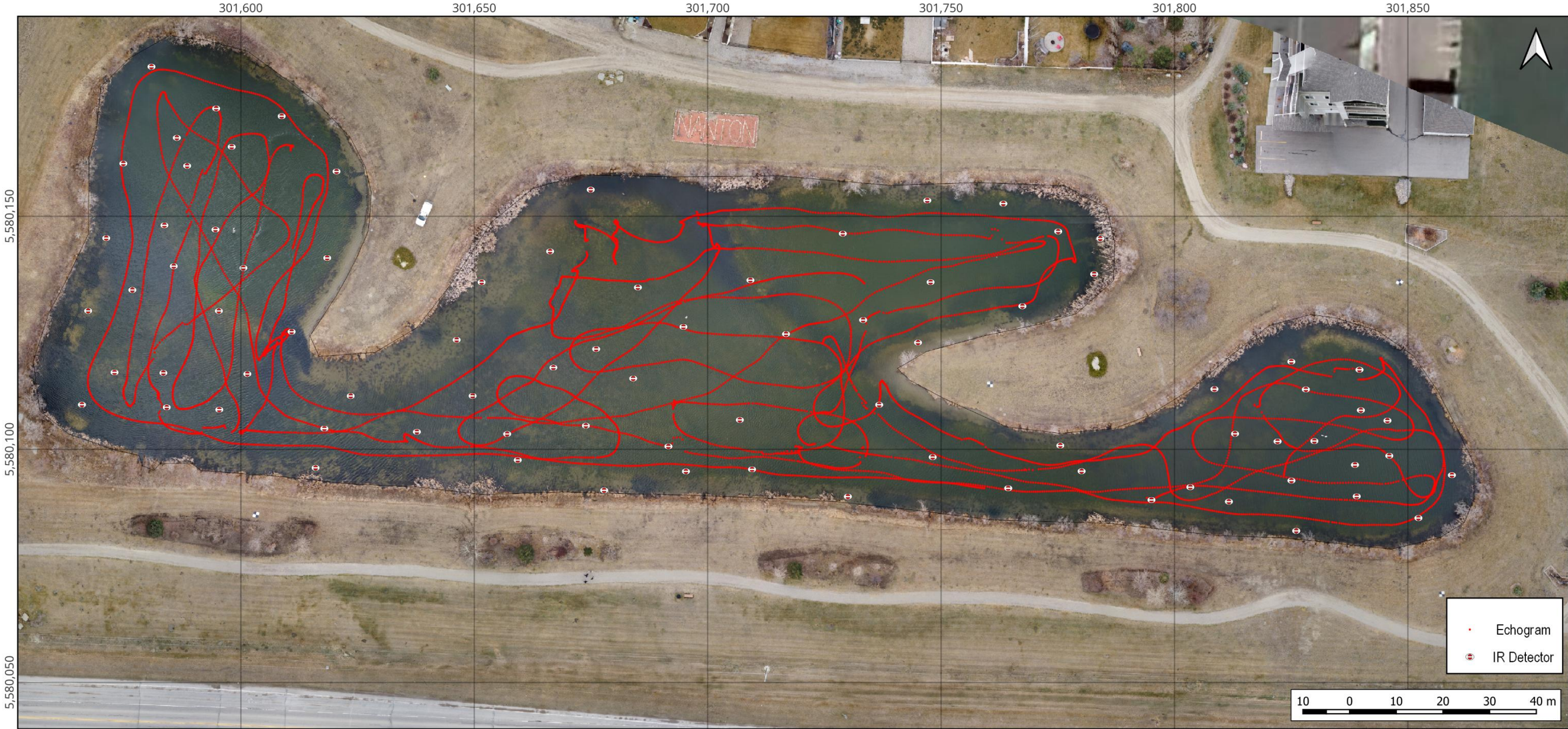
Figure 10 Westview Meadows Stormwater Pond raw survey lines & IR Detector measurements
