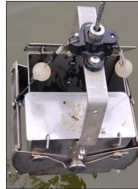
Figures 4 and 5 sludge sampler (left) and sludge sample collection (right) (sample images)
