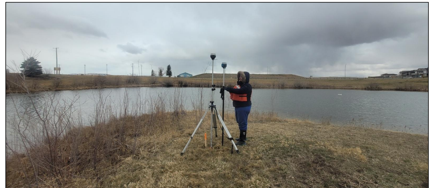
Figure 7 Hydrasurvey RTK base station setup over control point HCP1
